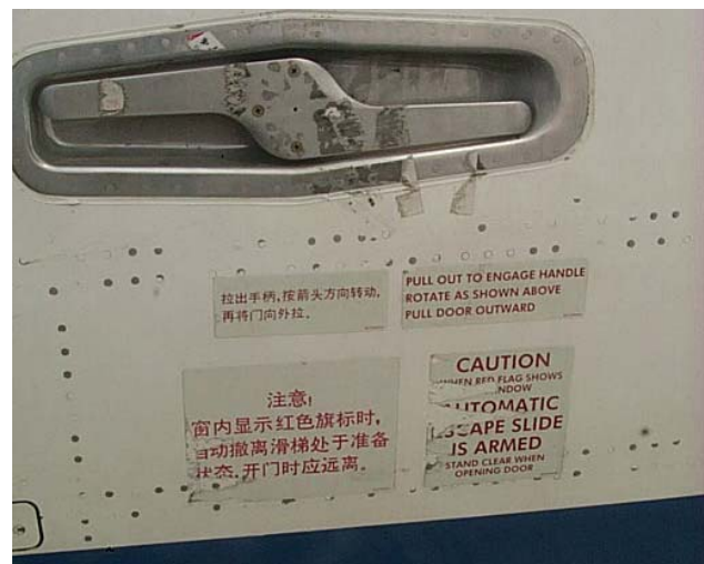
Figure 3. Rivet rash around door
