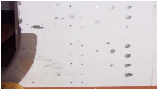
Figure 1. Rivet rash adjacent to forward airstair door
