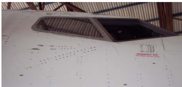
Figure 2. Rivet rash on fuselage structure
