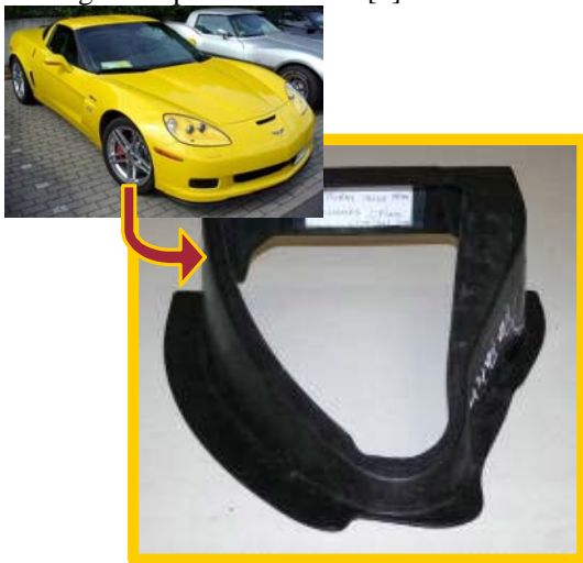
Fig. 7 – Corvette C6 Fender Well Component Molded from Recycled F18 Carbon Fiber [8]
