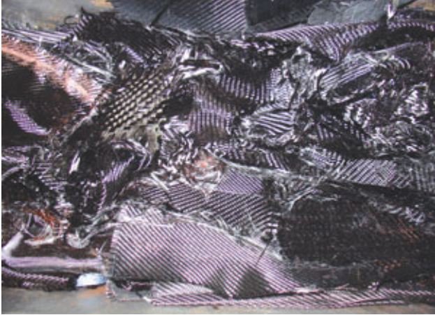
Fig. 3 - Scrap carbon fiber composite ready for shredding and fiber reclamation processing
