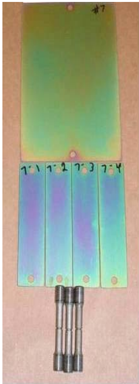
Figure 2 – Zn-Ni Test Specimens. 4 x 6” Corrosion Test Panel (Top), 1 x 4” Adhesion Test Strips (Middle), and ASTM F 519 Type 1a.1 Hydrogen Embrittlement Test Specimens (Bottom)
