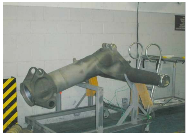
Figure 1 – Large complex high strength steel landing gear part that requires cadmium plating on external and internal surfaces.
