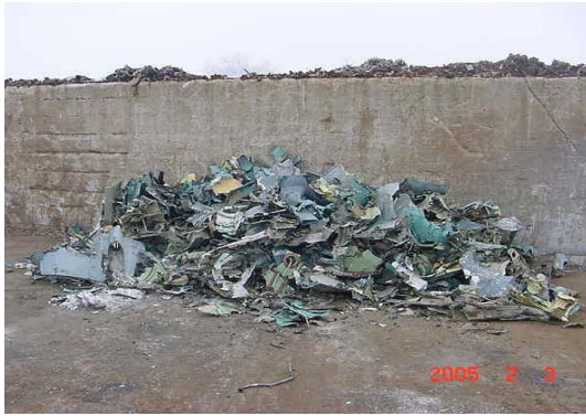
Figure 2 – Fuselage reduced to manageable size pieces for Fritz process*
