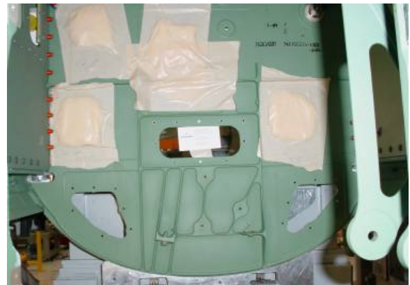
Figure 2 – Wet tape adhesion test patches on production subassembly.
