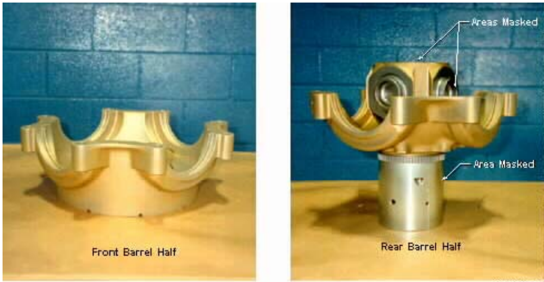
Fig. 3: C-130 Propeller Hub Barrel Halves IVD Aluminum Coated
