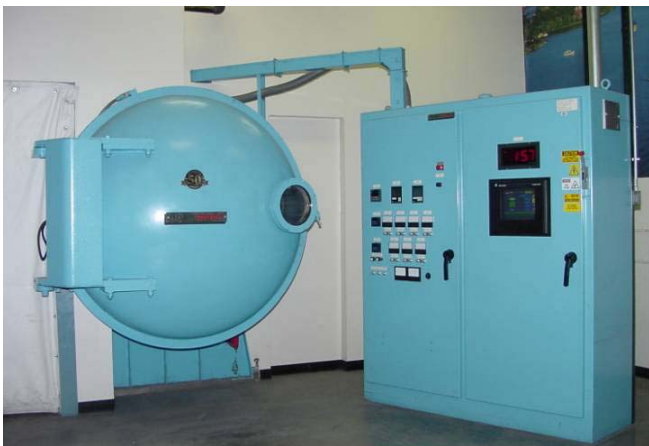
Fig. 1: Extended Length IVD Aluminum Coater at Boeing-St. Louis
