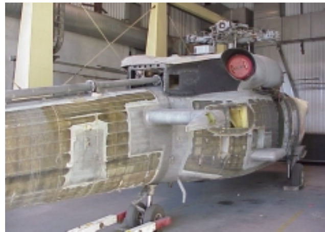
Figure 1. Portion of SH-60 Seahawk After Stripping
