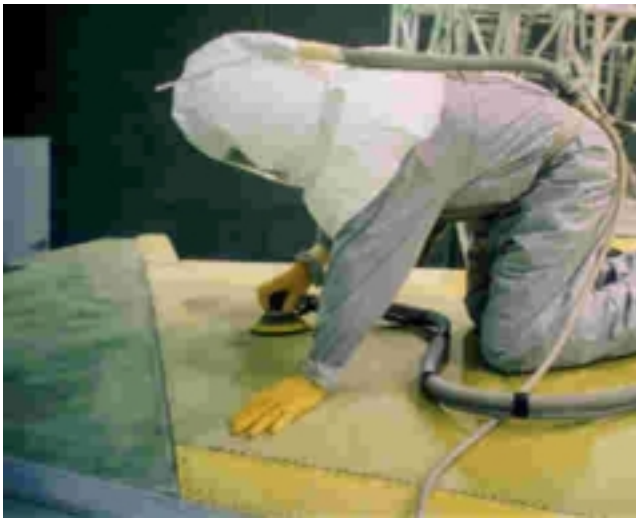
Vacuum-Assisted Sanding Operation
