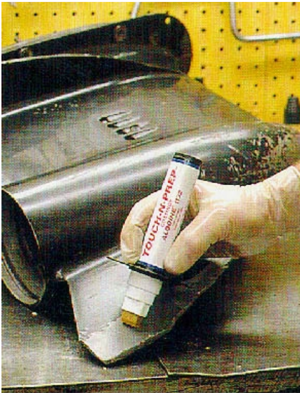
Preparation for Paint Touch-up
