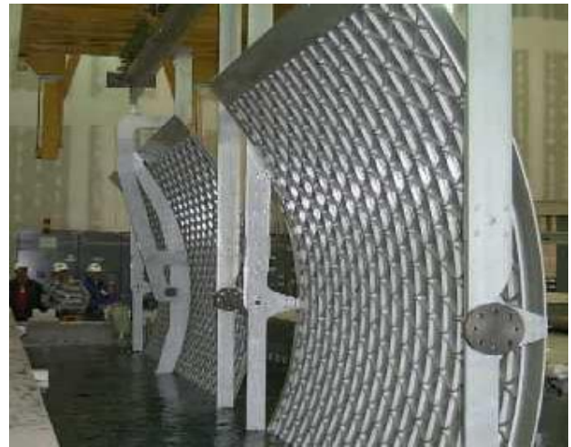
Fig. 6 Two skins mounted in tooling and ready for processing
