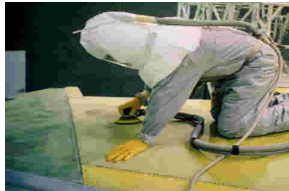
Fig. 4 –Scuff Sanding of Chromated Primers with HEPA Vacuum Engineering Control
